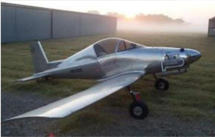
ards with a 19-foot wingspan and 15 foot length. At the empennage it looms to a whopping 6 feet tall. It is powered by an 1835 VW derived engine designed and assembled by Great Planes specifically for this plane. It is an all flush-riveted aluminum construction, though it could be assembled with pull rivets if preferred.
