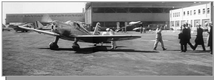
Scene from *The House Across the Bay*. Note the six exhaust stacks. This is the Ranger powered Model 1-C Aeroneer.
