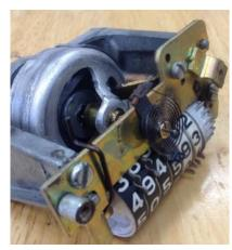
Photo 7: Front of Mechanism Showing the Calibrated Spring.
