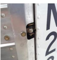
Photo 3: Installed Luscombe Rudder
