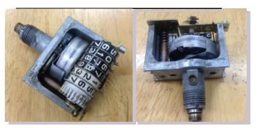
Photo 6: The Moving Parts of a Tachometer, Bottom View.
