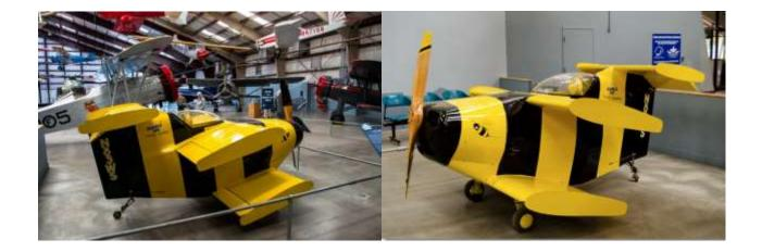
The Starr Bumble Bee was built to take a crack at the record for the world's smallest manned aircraft, with a 6'6 wingspan, a 9'4 length and a height of just 4'1. It took the Guinness record when it made its first flights in January 1984, and was capable of speeds up to 180 mph, but could only fly to a service ceiling of 3,000 ft due to its tiny wings. From: New Atlas. March 25, 2019
