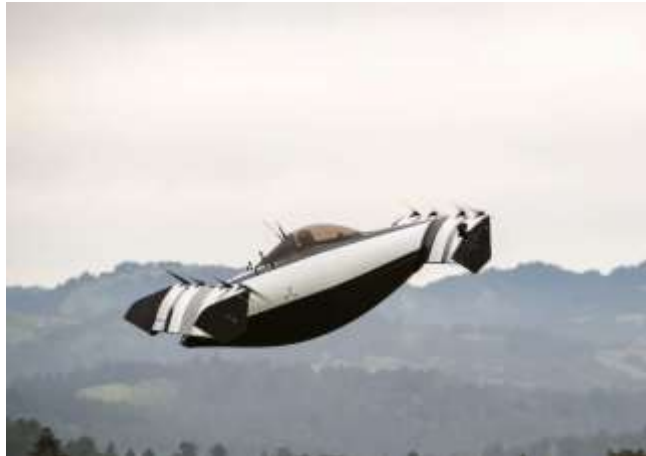
BlckFly is a single-seater electric VTOL aircraft (Credit: Opener) From: New Atlas, December 27, 2018
