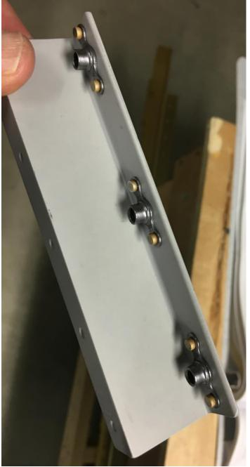
A z-bracket with nutplates installed.
