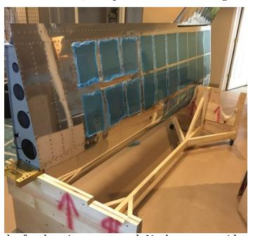
the fuselage is constructed. Van's even provides a drawing. This task is a chore because my carpentry skills are, ahem, rough. I had to purchase only 4, 2x4s from Lowes and 4 casters from McMaster-Carr. The rest of the structure was the shipping crate from Van's that once was full of wing components. All the wood screws were left-overs from other projects.
