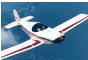
Rand-Robinson Engineering KR-2 Two seats, trigeared or tailwheel, 1000 hours, 1250 flown, C, W $8500
