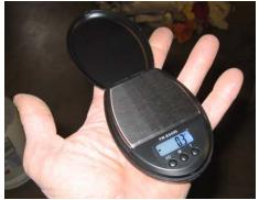
racy is quite good. It measures down to one tenth of a gram. It has a tare weight button so I can place a square of cardboard on the scale and then zero it out. I put on about 40 grams of sealant, then add 4 grams of accelerator and then mix it up. With the balance, I could do the same thing, but I then had to remove the sealant and accelerator from the two trays and place them together on cardboard and then mix. The new scale was much quicker.
