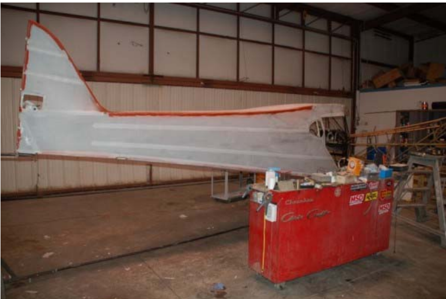
clear coating the fuselage
