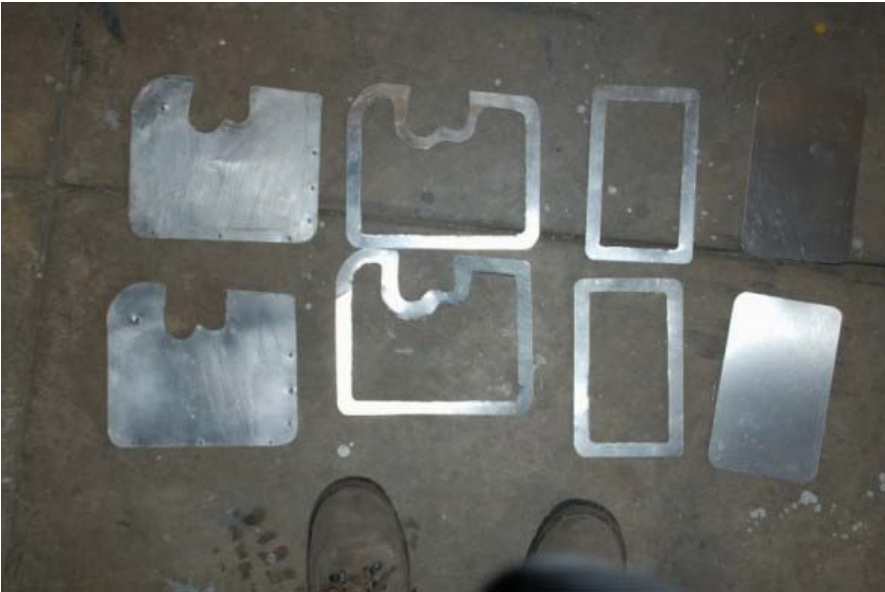
Made new aluminum inspection frames
