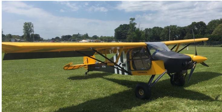
The fabric covering is made of Oratex. It's pre-painted, pre-colored, UV protected, and very lightweight. Covering is a one-step process: you glue it on the frame and you shrink it.
