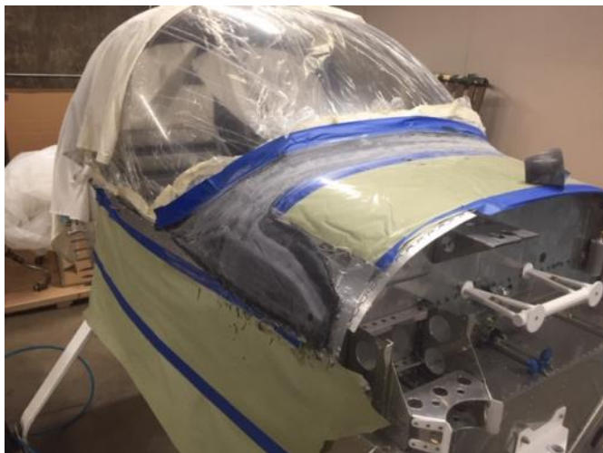
Fiberglassing the canopy frame.
