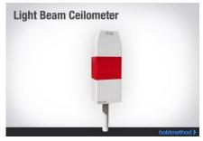
cloud height. CHI is normally limited to 12,000 feet of altitude, which is why you'll sometimes see "clear below 12,000 feet" in a weather report. CHI is the most common cloud measurement device used at airports today, and with technological advances, it will soon allow cloud measurements up to 24,000 feet.
