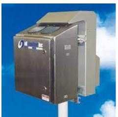
3) Cloud Height Indicator (CHI) Sensors use vertically pointing lasers (LIDAR) to measure cloud heights. You can think of CHI like radar; the round trip time for the beam to return once hitting a cloud layer determines
