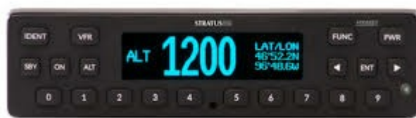
An ADS-B transponder with Lat/Long read-out, showing that the position source is working.
