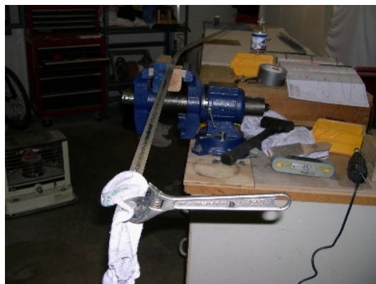
(Right Hand Longeron bending. Notice the deadblow mallet on the workbench)
