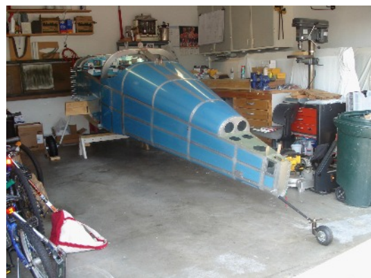
(Fuselage structure close to being finished. Between the work bench and the wall you can see the wings wrapped in old bed sheets)
