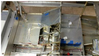
Having nearly completed the fuselage and wing kits, we got started on the Finishing Kit. It comprised of wiring harnesses, tubing for fuel lines, upper and lower cowling, landing gear and fairings, wheels, canopy and its structure, and a number of other small parts. Bob M. took the gear fairings home and started work on them. This involved some cutting and fine tuning the fiberglass
