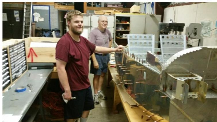
Once everything seemed to fit, the roll bar was installed along with the baggage bulkhead. The removable avionics cover was completed and fastened in place. It's really starting to look like an airplane now. Some people call this the boat stage.
