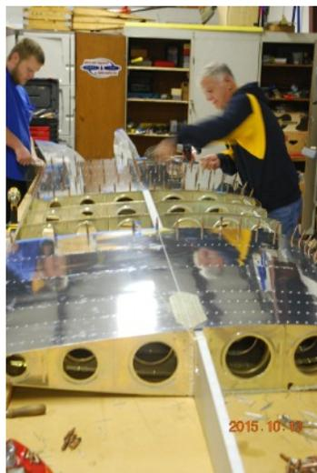
There are a lot of rivets involved in putting the skins on the wings. This is a fun part, as when you're done, it really does look like an airplane wing. Pneumatic riveting tools make quick work of the riveting process. Skinning the wing only took about an hour. Bottom skins went on first. We then carefully flipped the wing over and installed the top skins.
