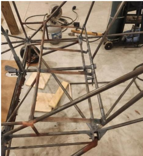
I got to work making a new horizontal seat bar and then made a vertical tube coming down to support the down pressure of the occupant(s). Then I needed to figure out how to hold the wooden seat. I bent up some 1-inch strips on 1/8 inch 4130 plate into “L” brackets and welded them on the back seat tube. This allowed me to drop the seat pan even lower as I needed the headroom beneath the top longeron. I then welded in tabs on the front seat support horizontal.
