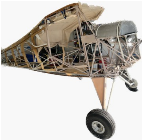
Figure 2 Chief fuselage with headliner installation
