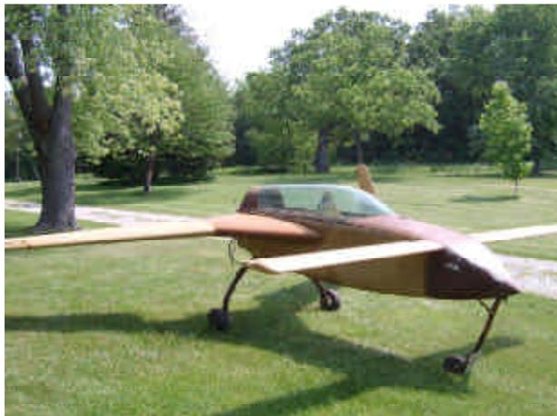
The engine is a Continental c-90, with new bearings, rings, reworked 0-200 cylinders, gaskets, starter, and generator. It needs magnetos and final assembly by either the buyer or a certified tech. The plane has a Long Eze landing gear, airbrakes, electric aileron trim, manual elevator trim, and engine cowling. All controls are installed. If you have any further questions please contact me at 618-488-7471 (Sorento, IL).
