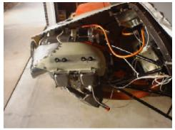
Photos: Opposite page, fuselage sitting on mains; Jabiru engine installation
