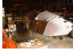
three ways: either a complete kit, a components kit, or the "scratch build" kit (Gary's choice). From the factory, Gary purchased hard to build things like the cowling, canopy, and some metal parts. He also got forming blocks and a really good set of plans. Anybody who buys a set of Sonex plans is also entitled to a complimentary 2-
