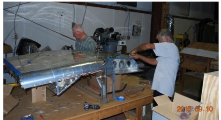
Once the bottom skin was secured, the lower firewall was installed. By now the fuselage has its full length from baggage compartment forward to the firewall. The
