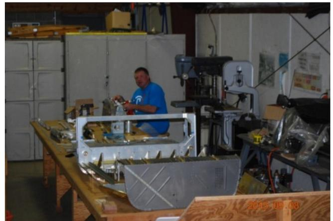
the fuselage structure. We all are amazed at how the fit and quality of the prepunched sheet metal parts are. For the most part, one simply cleco's the parts together and then rivets them. In a few cases small parts need to be made and match drilled to their mating part. Vans really does a great job making things line up.
