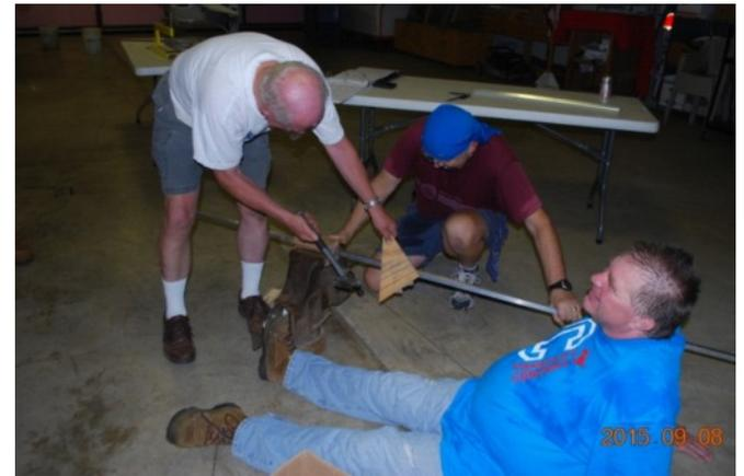
member Chuck started that process out by installing nutplates onto the sheet metal. Then we turned the fuselage section upside down and started clecoing the skin to the frame.
