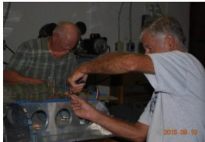
Hundreds of rivets later, the skin was attached. The process of pulling the rivets took about 15 minutes with 5 people working on it. It was really busy for a while, sounding like an aircraft factory in full swing.
