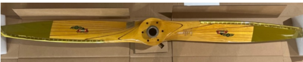
Overhauled Chief Propeller Back From Sensenich
