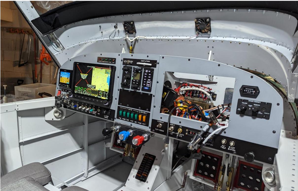
Instrument panel under construction. In this photo the panel was powered up.
