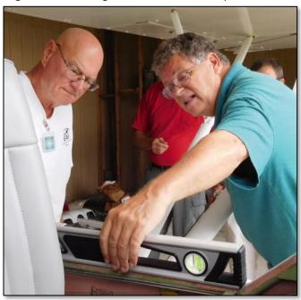
measuring the distances from there to the center of the main and tail wheels. These distances are as important as the three weights when calculating the aircraft center of gravity.
