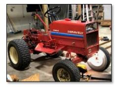
a result pertinent to the conversation. Well, of course, after being immersed in water, it would not run. He completed a complete replacement of the electrical system and he is happy to report that the tractor is now up and running again.
