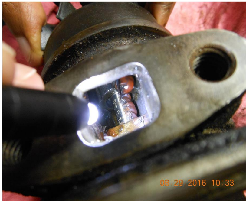
Photo 5 – View of foreign material in center turbo housing
