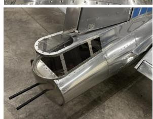
The engines are rated at 80 hp, but with no room for a prop speed reduction unit in the scaled-down cowlings, the engines are connected directly to the propellers, resulting in 60 hp at 3300 rpm, or a total of 240 hp. They burn about 4 gph each, for a total of 16, sipping from two tanks in the wings with a total capacity of 40 gal-
