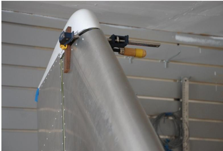
*Figure 2: Rudder clamped into the centred or neutral position and aligned with the tail fin and aircraft centre line along the top of the fuselage.*
