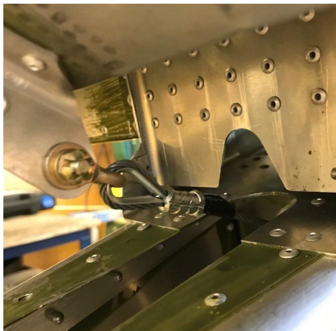
*Figure 11: Lower elevator cable and shackle attachment to the lower elevator horn.*
