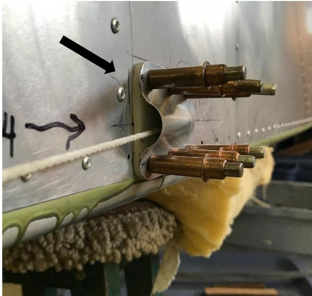
Figure 3: Rudder cable exit fairings have 2 components, a Delrin plastic insert (arrow) that the cable slides through and is protected from the fuselage sheet metal at the exit slot and the aluminum fairing. Initially a string was used to position the fairing relative to the cable position.
