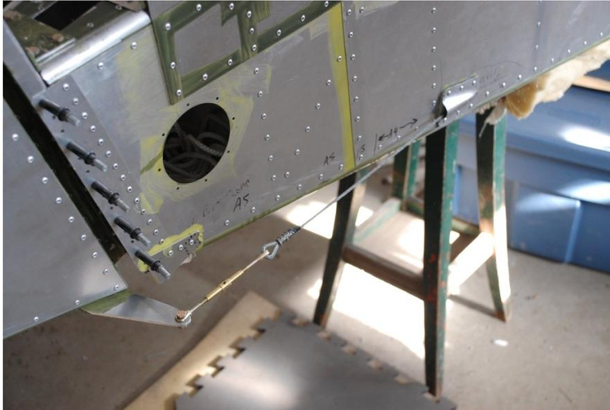
*Figure 5: Cable and turnbuckle at rudder horn.*
