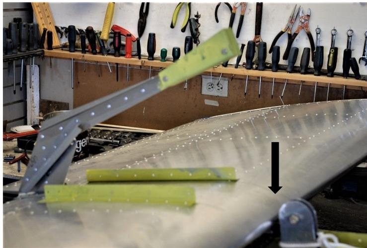
*Figure 9: Weights (in green primer paint) were attached to elevator upper arm to achieve static balance. This will change slightly after painting and final adjustments can be made before the tail fin forward fairing is riveted in place. The cable pulley is just forward of the stabilizer leading edge (arrow).*
