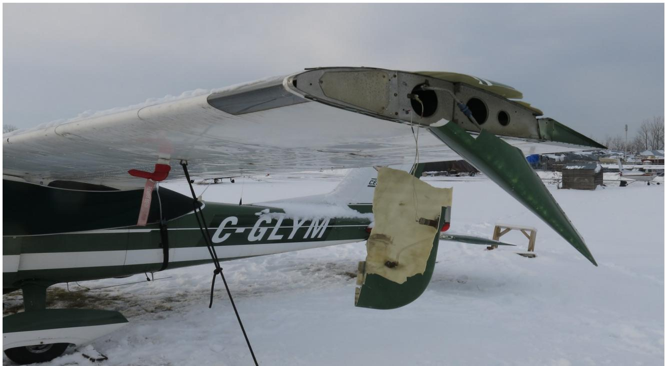
*Figure 3: Damage to left wing*
