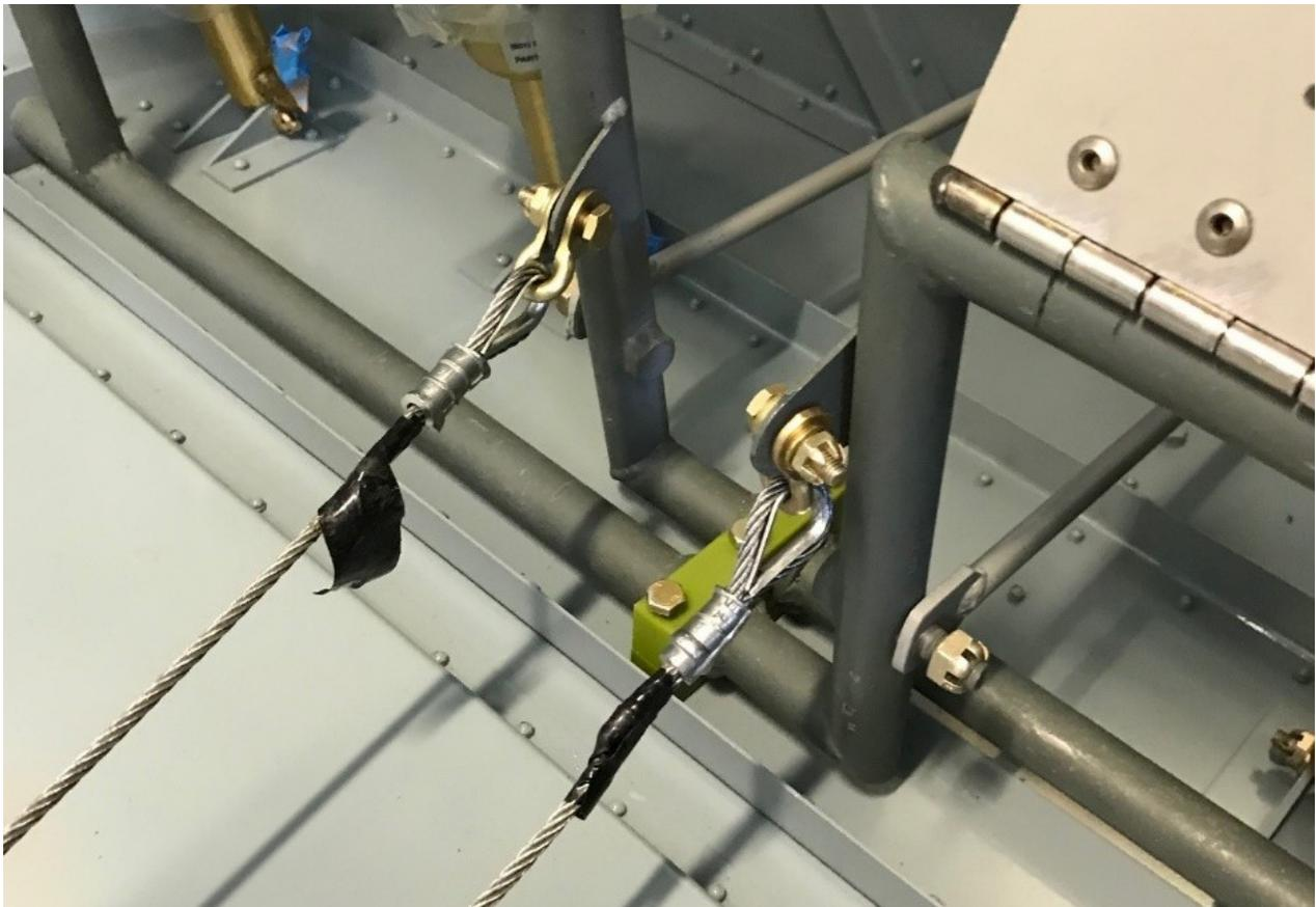
*Figure 6: Rudder cables and shackles at the pedals.*
