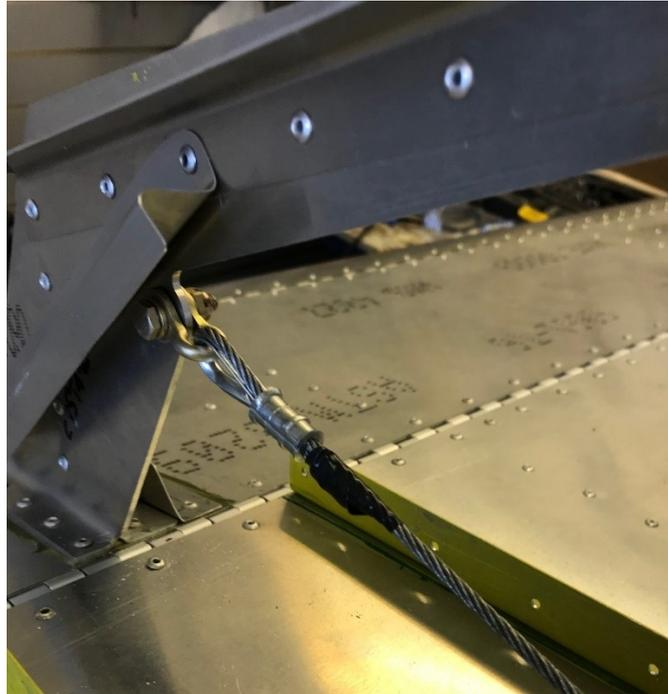
*Figure 10: Upper elevator cable attached with a shackle at the upper elevator arm.*
