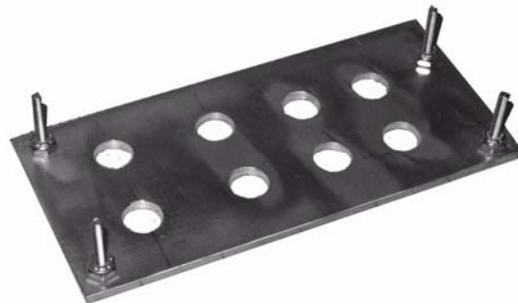
mounting tabs will fit down over the screws. Nuts can be tightened down to secure it. For a composite aircraft installation, the bottom of the plate (shown above) should be flocked and the holes in the plate filled with flock before applying fiberglass layers over it to secure it to the fiberglass structure.
