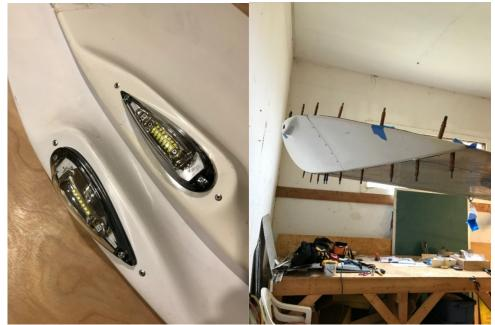
AVEO Engineering LED wingtip lights were acquired and fitted to the plastic wingtips. The wingtips were fitted to the wings and drilled ready for riveting. The lights were installed so that they can be removed as their own inspection panels to access wiring connections just
