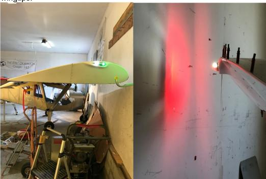
And finally, the big question – do the lights work? The wiring connections and lights were tested at stages during the installation and for this a 12V battery from a cordless drill was used as the power supply. The strobes give an intensely bright flash even during daylight and are built in with the navigation and position lights.
