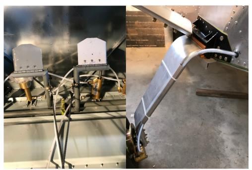
The Cruzer has dual brakes and brake lines were fitted using tubing specified by Matco for their brake assemblies. Brake lines were routed to exit the fuselage at the sides just behind the main gear attachment brackets and then follow trailing edges of the gear legs to each caliper. A metal protective shroud was temporarily secured with zip ties.
