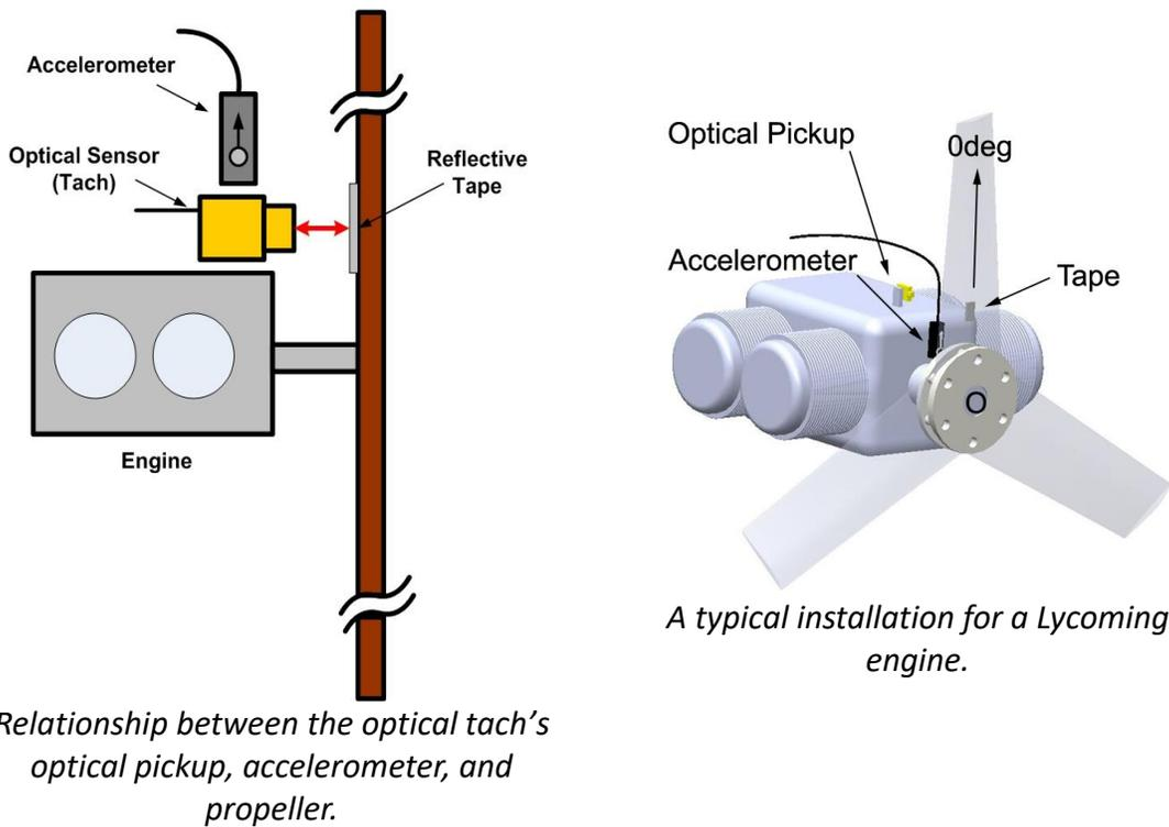
The optical tach's optical pickup should be at least six inches from the reflective tape, but not so far that the optical tach cannot obtain a reading from the tape.
