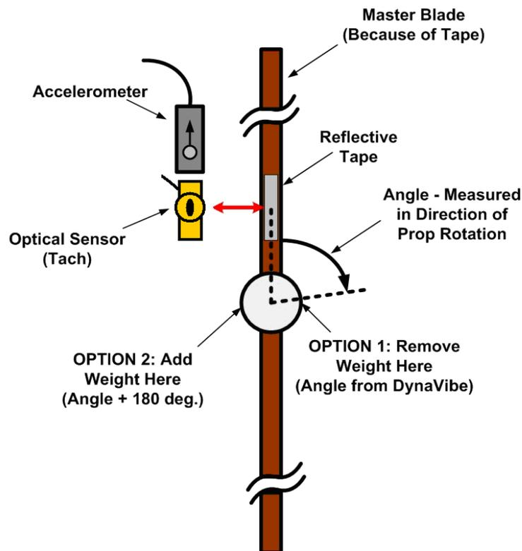
*Showing the phase angle relative to the master blade.*
