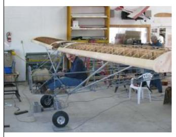
The J3 Kitten is a high wing 3/4 scale J3. It is made up of traditional construction just like the original J3. Chromoly frame, wood wing covered
