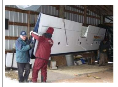
Today we put the wings back on Andre Girard's Titan Tornado. Luckily the temperature was mild. The Titan had a small transformation done to it. A heater and hydraulic skis were added, and the engine motor mount was reinforced as per an AD from
