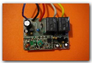
Photo 3 Top of the wireless control board
