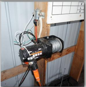
Photo 1 12V winch with starter relay on top
