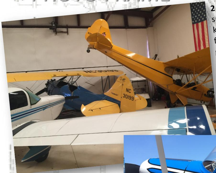
**2 in 1.** Firstly you save space. Secondly, small engines (Cub, Aeronca, etc.) are known to lose oil pressure when parked for a long time. This way of parking will give you a good oil pressure reading on your next start!
