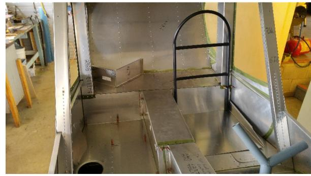
dimple the holes and then rivet on the nutplates with flush rivets. We also learned how to use a tool to install rivnuts to allow easy access to the area under the centre console, another enhancement we had decided on.
