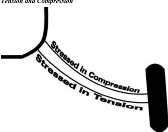
When we think about applying stress to a metal part, we usually think in terms of tension -- in other words, applying a load that tries to pull the metal apart. Cylinder studs and crankcase through-bolts are examples of metal parts that are loaded in tension. Aluminum alloys may have tensile strengths between 20,000 and 80,000 PSI, while high-tensile-strength steel can withstand 200,000 to 400,000 PSI or more.
