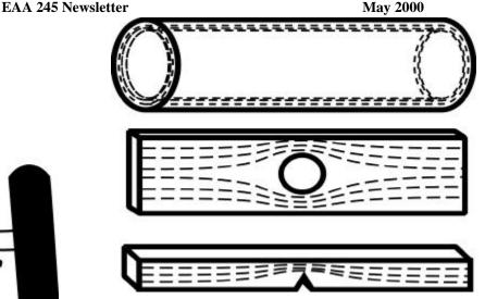
When a metal part is placed under load, stress is almost never uniformly distributed through the part. Instead, it concentrates in certain areas. Naturally, those areas of stress concentration are where the part is most likely to crack or fracture.
