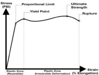
Consider what happens when you apply force to a piece of metal: It deforms. The force you apply is called stress, and the amount of resultant deformation is called strain. The relationship between stress and strain is what defines the structural properties of the metal. (See Figure 4.)
