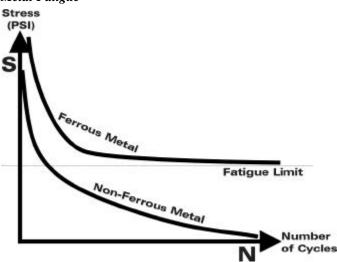
Take an ordinary paper clip, straighten, and then bend it back and forth repeatedly until it breaks in two. What happened? You just demonstrated metal fatigue.
