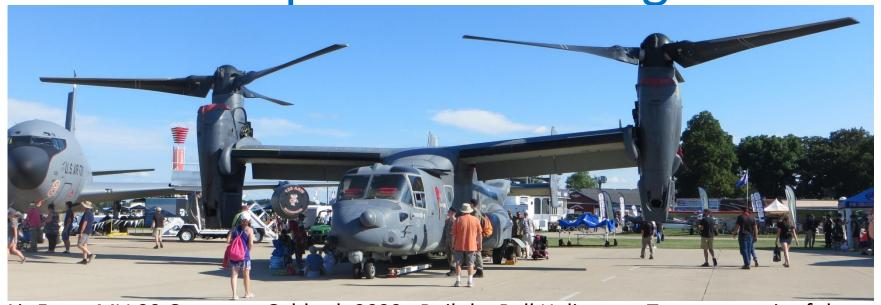
Air Force MV-22 Osprey at Oshkosh 2022. Built by Bell Helicopter Textron, a unit of the Boeing Corp. The Air Force has 54 in Special Operations Command. Two RR Liberty 6200 shaft HP engines, top speed of 280 knots. Crew of 4, armed with 1.50 cal MG on ramp.
