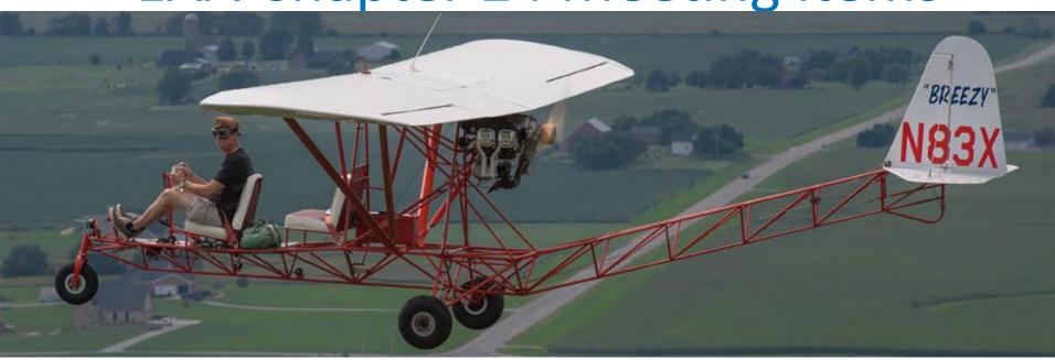
A Breezy homebuilt. Wings are from a Piper super cub as are the three seats. First flew in 1964. Engines is a Continental C-90, 90 HP. About 1000 have been built in various mods.
