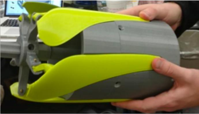
Prototype for the high lift motor folding propellers.
