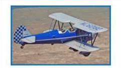
SERV-AERO SUPER STEARMAN R-985-14B P&W; 22D-30 HAMILTON STANDARD ALDIN QUICK DRAIN TO PREVENT HYD LOCKS NEW STAINLESS EXHAUST-AIR WOLF OIL FILTER INVERTED OIL & FUEL-FOUR AILERONS WITH
