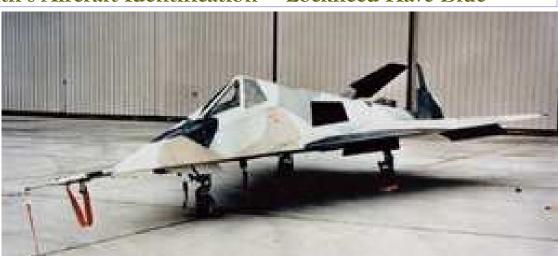
To design the aircraft, the Skunk Works' design team leveraged the mathematics published by Soviet physicist and mathematician Petr Ufimtsev regarding the reflection of finite analysis of radar reelectromagnetic waves. A flection.
