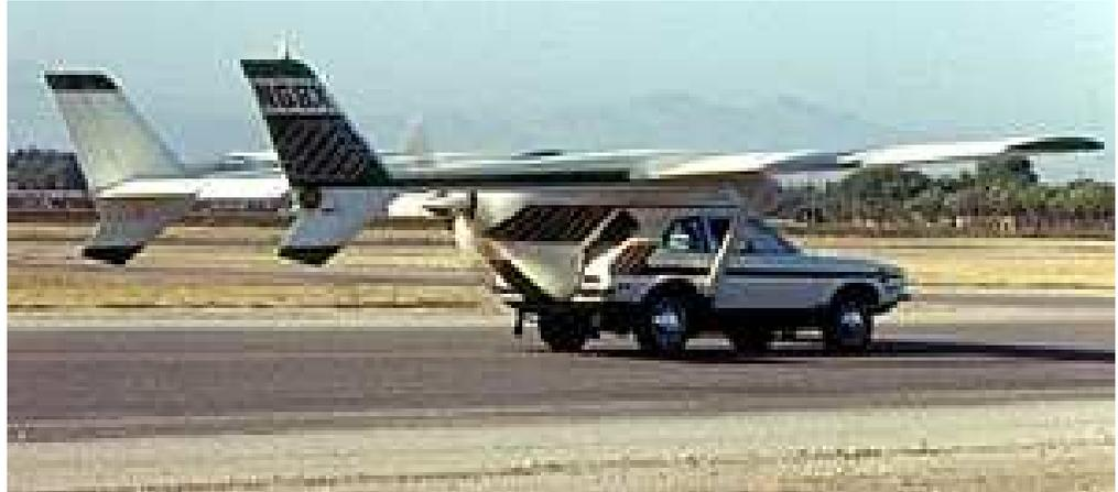
The Mizar was intended to use both the aircraft engine and the car engine for takeoff. This would considerably shorten the takeoff roll. Once in the air, the car engine would be turned off. Upon landing, the four-wheel braking would stop the craft in 525 ft (160 m) or less. On the ground, telescoping wing supports would be extended and the airframe would be tied down like any other aircraft. The Pinto could be quickly unbolted from the airframe and driven away.
