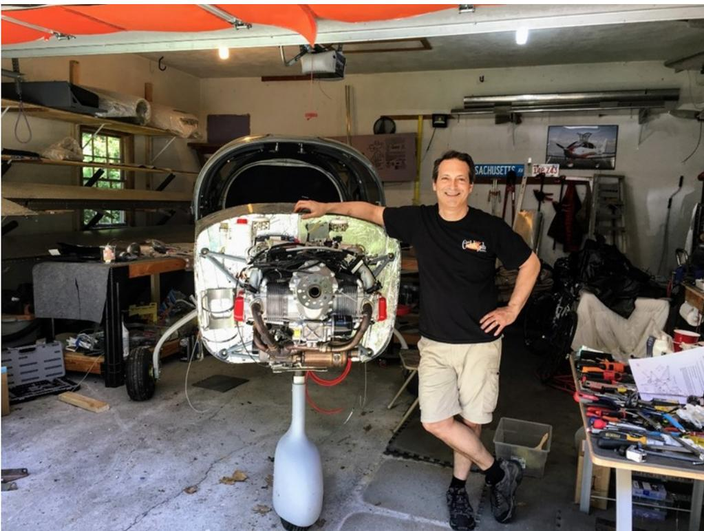
With the canopy on and the dash positioned, it was nearly an airplane. Lots of work on the interior and then the firewall (charging/starting circuits) was done at that point and then it was time to install the engine. I rented a ridiculously oversized engine lift and it went on without much difficulty.
