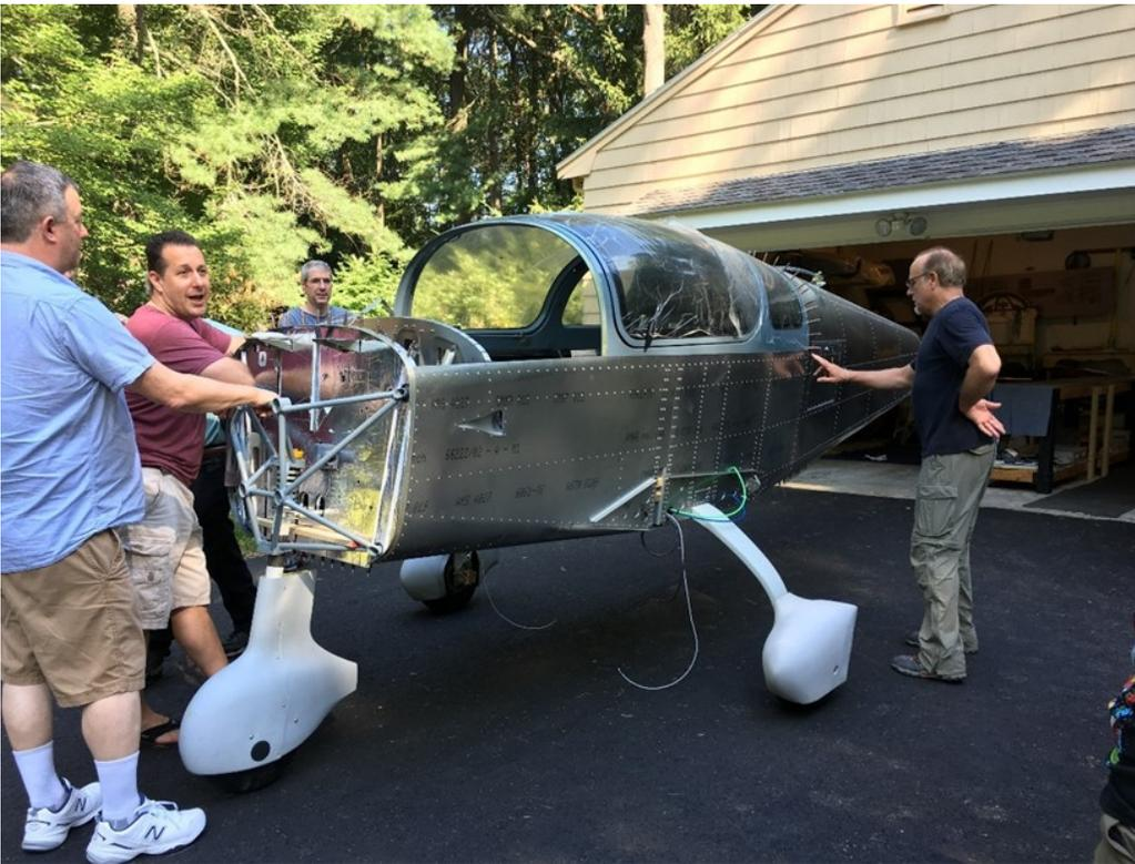
*Installing the massive fiberglass landing gear was difficult, but I was able to put it on its wheels, which was a huge milestone.*
