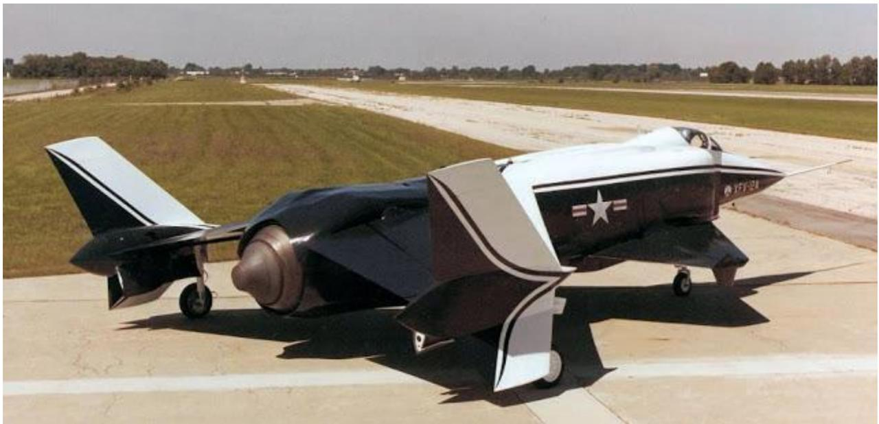
The XFV-12 design attempted to combine the Mach 2 speed and AIM-7 Sparrow armament of the McDonnell Douglas F-4 Phantom II in a VTOL (vertical takeoff and landing) fighter for the small Sea Control Ship which was under study at the
