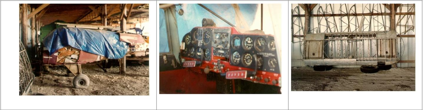
Converted parts and plane to tail dragger & Ford power...Bought three wrecked wings to make two good ones.
