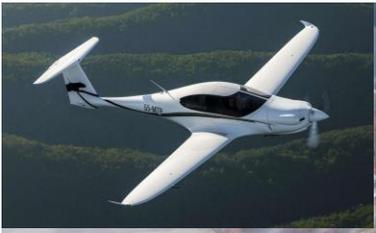
This picture is a Pipistrel Panthera, a lightweight, all-composite, highly efficient four-seat aircraft by Pipistrel of Slovenia. The petrol-powered version of the Panthera, powered by a Lycoming IO-540, is intended to cruise at 198 KTAS at FL 080 for over 1,000 nm with a 14.8 gph fuel burn.
