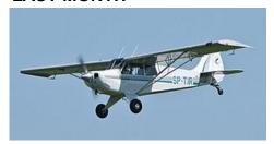
This picture is the Aviat A-1 Husky, a tandem two-seat, high-wing, utility light aircraft built by Aviat Aircraft of Afton, Wyoming. The aircraft was introduced in 1987, and has been used for observation duties, fisheries patrol, pipeline inspection, glider towing, border patrol and other utility missions. The aircraft max gross weight is 2200 pounds, powered by a Lycoming O-360-I1P, with a fuel capacity of 50 gallons. For more information, visit https://aviataircraft.com.
