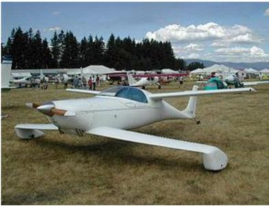
The mystery aircraft to the left is a **Quickie Q2**, a 2-seat version of Rutan's Quickie. This aircraft has a 64-horsepower Volkswagen air-cooled engine. The prototype first flew in 1980. Over 2000 have been built.
